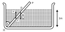
Then  $OC = \frac{OD}{2} = \frac{1}{2} \sec \theta$ . If A is the area of cross-section of rod, then mass of rod
